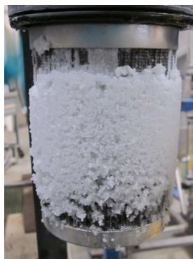
Figure 2: Clogging of a typical fuel filter [29].
