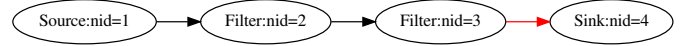
Fig. 4: The source produces taxi ride items then they are filtered in order to get statistics on the rides in New York city (e.g., rides that have not started, rides taking too much time) and eventually stored in a Kafka topic.
