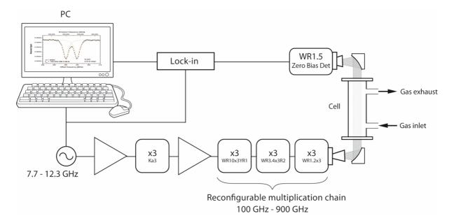
Figure 1. Frequency multiplication spectrometer shown with an overall multiplication rank of  $\times$  81 able to cover 630 GHz to 900 GHz.
