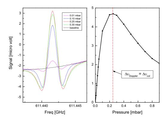
Figure 3. Left pane, spectra of a calibrated 50 ppm trace  $H_2S$  in  $N_2$ , recorded with a modulation depth of 1188 kHz, an interaction length of 1.128 m, and at a temperature of 293 K. Right pane, signal amplitude as a function of the working pressure, maximum value when the collisional broadening matches the Doppler linewidth.
