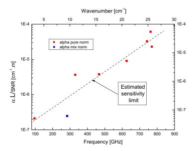
Figure 2. Estimation of the minimum detectable absorption coefficient  $\alpha_{min}$  as a function of frequency for an interaction length of 1m. All values are for a measurement bandwidth of 1 Hz. Red
