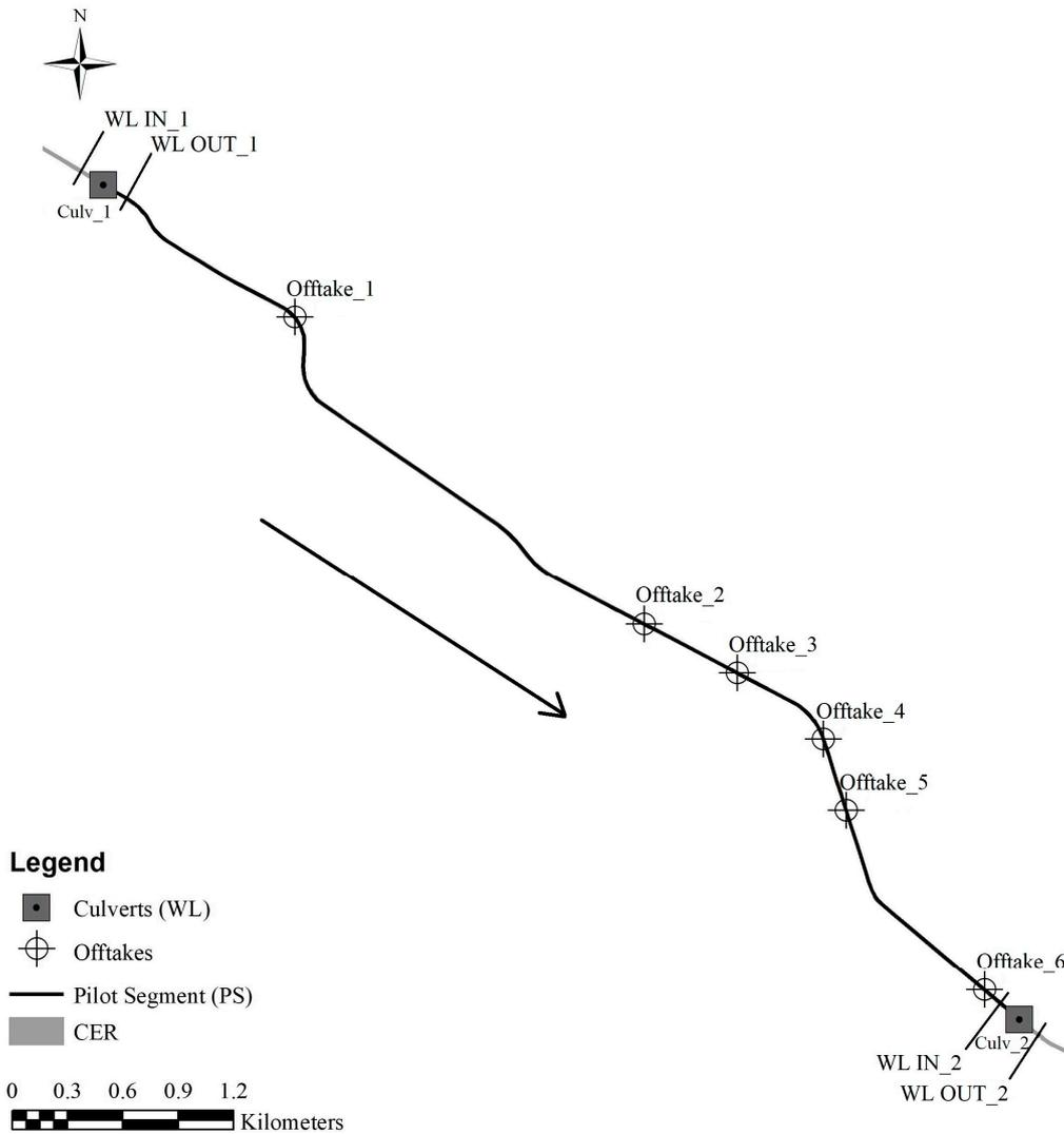
**Figure 2.** The scheme of Pilot Segment (PS): The six irrigation offtakes, the two culverts passing under the Idice River (Culv\_1) and the Quaderna River (Culv\_2), the four water gauges (WL) at the IN and OUT of both the culverts.
