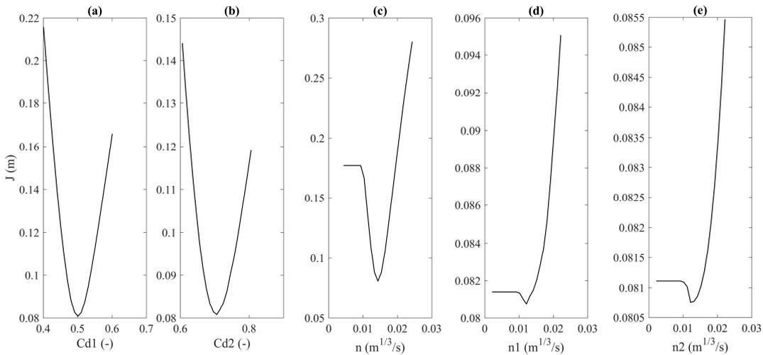
**Figure 4.** For 2015,  $Cd1$  (a),  $Cd2$  (b),  $n$  (c),  $n1$  (d),  $n2$  (e), the cuts of  $J$  around the minimum values of the parameterized hydraulic variables. In all cases they represent real minimum for the criterion.
