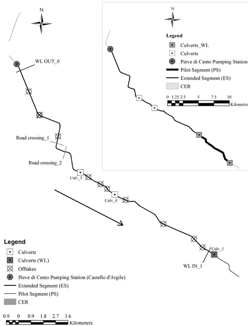
**Figure 5.** The scheme of ES: The 12 irrigation offtakes, the three culverts under passing the Idice River (Culv\_1), the Navile Canal (Culv\_3), and the Savena River (Culv\_4), the two water gauges (WL OUT\_0 and WL IN\_1) at the OUT of the pumping station Pieve di Cento and at the IN of Culv\_1, the two road crossings.
