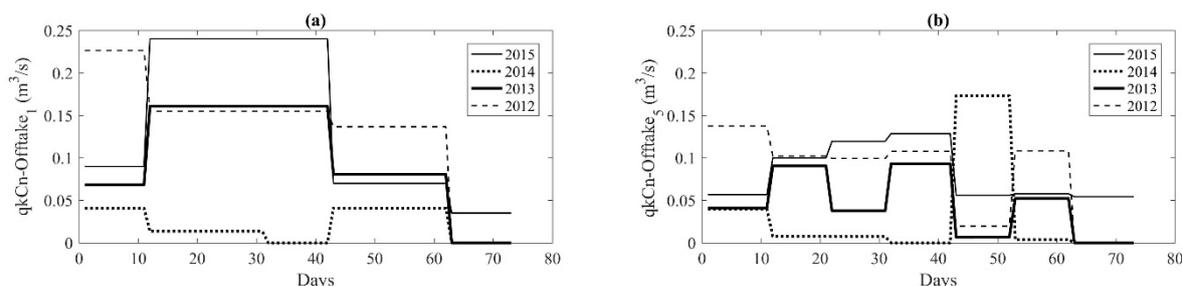
**Figure 7.** For every year, the variability of the diverted discharges for the reference offtake (Offtake<sub>1</sub>) (a) and for a generic offtake (Offtake<sub>5</sub>) (b).
