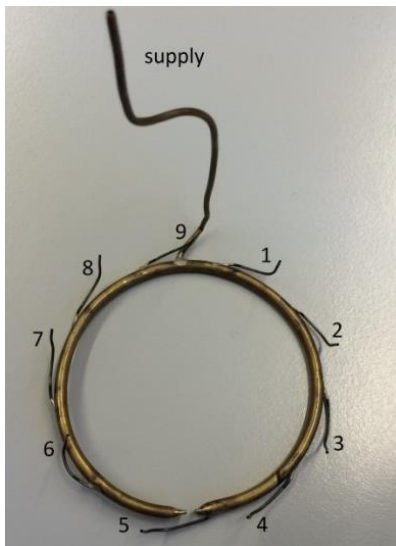
Figure 3. Fuel distributor with designation of the fuel injections
