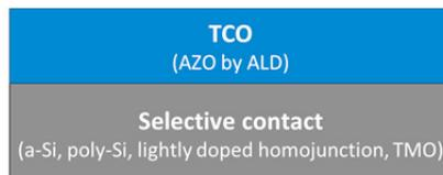
Fig. 1. Schematic diagram of the positioning of the TCO layer developed for passivated contact purposes.
