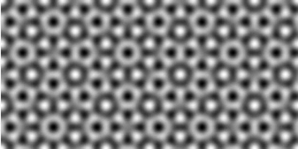
Figure 1: Example 8-fold quasipattern. This is an approximate solution of the Swift–Hohenberg equation, see [11].
