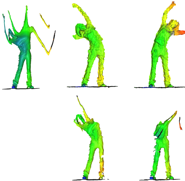
Figure 7: Failure case: large motion are not handled well by our method. Left: Lidar Scan. Depth sensor frames (top row) and corresponding corrected frames (bottom row).
