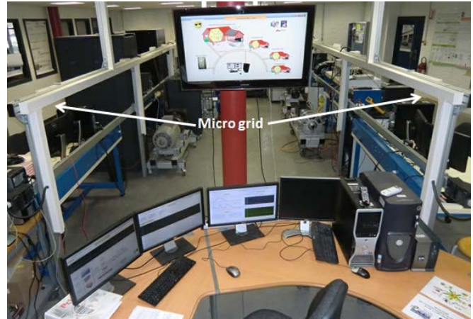
Fig. 10. Overview of our SCADA system.
