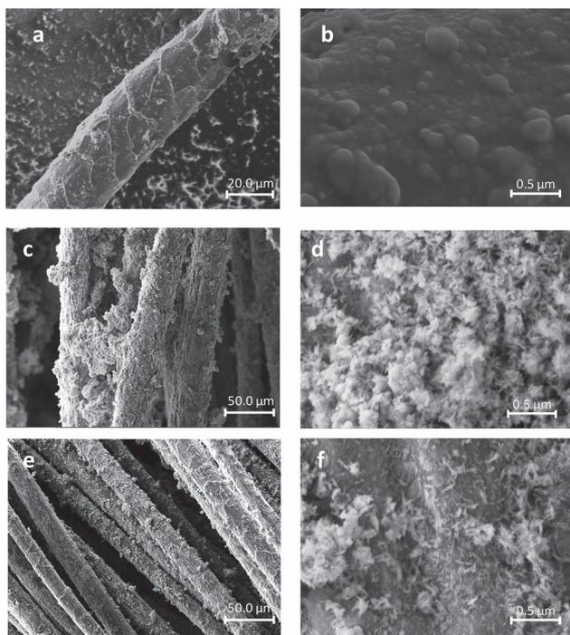
**Fig. 6** SEM pictures of wool fibers coated by PPy mineralized with TiHA25. Surface of the WAP fibers after mineralization at increasing magnification (a and b); surface of the WEAP5 (c and d) and WEAP10 (e and f) fibers after mineralization at increasing magnification.
