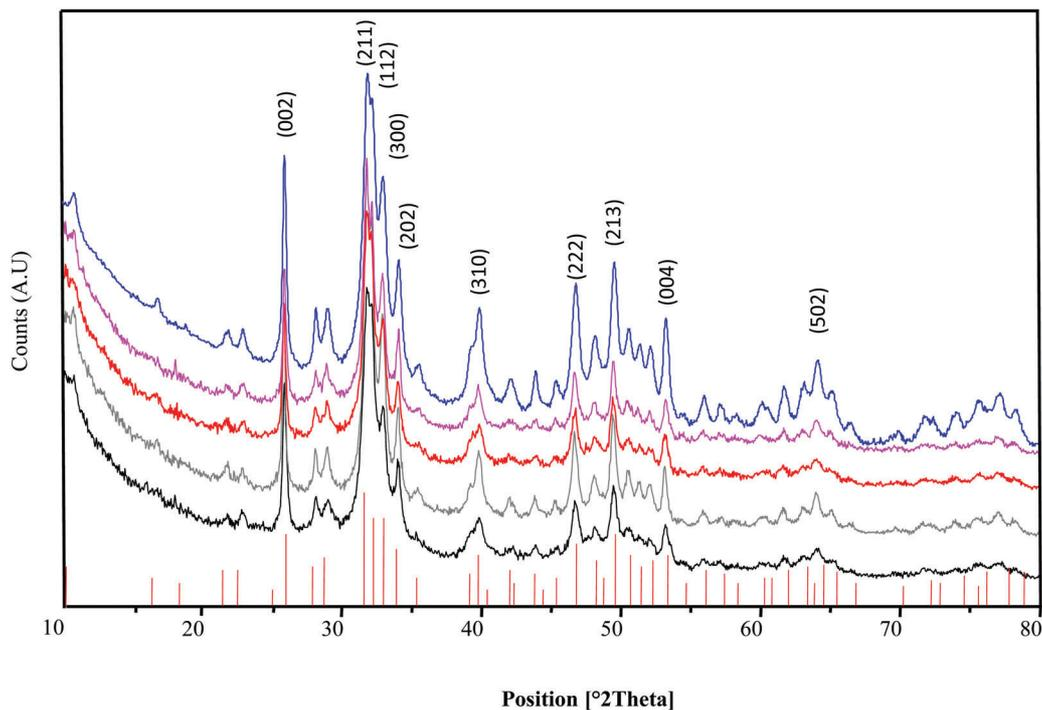
Fig. 1 XRD diffraction patterns collected on (from the top to the bottom) HAp, TiHA50, TiHA25, TiHA17 and TiHA8.
