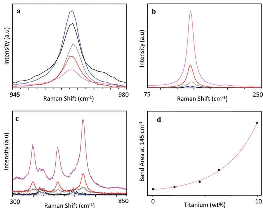
**Fig. 3** Evolution of the Raman bands of apatite (a) and anatase (b and c) of thermally treated HAp (blue), TiHA8 (black), TiHA17 (grey), TiHA25 (red), and TiHA50 (violet), together with the curve obtained by plotting the area of the Raman band at  $145\text{ cm}^{-1}$  registered on all the TiHAs as a function of their Ti concentration (d).
