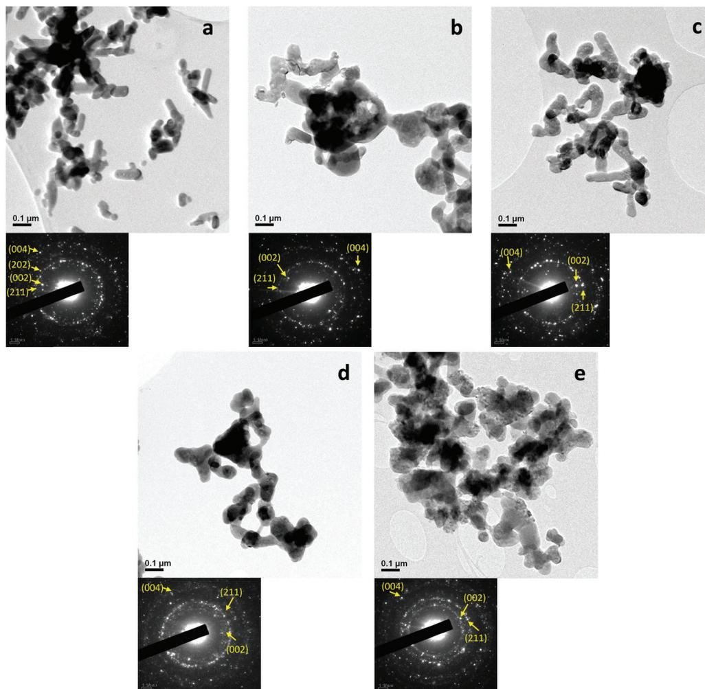
Fig. 4 TEM pictures and SAED patterns collected on samples HAP (a) TiHA8 (b) TiHA17 (c) TiHA25 (d) and TiHA50 (e).
