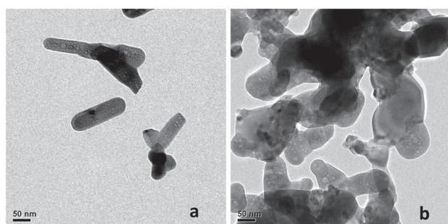
Fig. 5 TEM pictures of HAP (a) and TiHA (b) at high magnification showing NPs nanopores.
