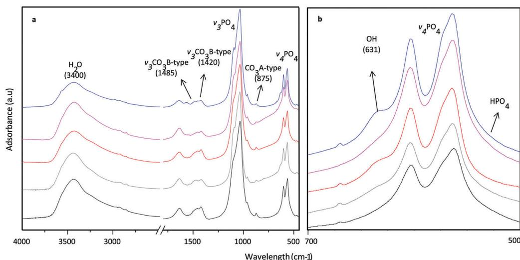
Fig. 2 FT-IR spectra of (from the top to the bottom) HAp, TiHA50, TiHA25, TiHA17 and TiHA8 (a). Magnification of the FT-IR spectra in the region where the bands of  $\nu_4PO_4$  ( $675\text{--}525\text{ cm}^{-1}$ ) appeared (b).
