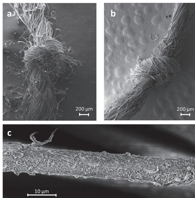
**Fig. 7** SEM pictures of knotted WEAP5 yarns before (a) and after (b) bio-inspired mineralization, with a micrograph of mineralized WEAP5 after dipping at 40 °C in ethanol for 15 minutes (c).
