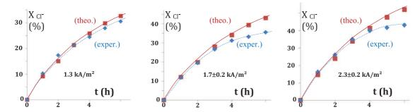
Fig. 8. Comparison between theoretical ■ and experimental ♦ 'temporal evolution of the chloride conversion for galvanostatic electrolyses conducted, under three current densities.  $V_{\text{anolyte}}$ : 150 cm³;  $V_{\text{catholyte}}$ : 90 cm³;  $V_{\text{catholyte}}$ : 90 cm³;  $V_{\text{f assumed}}$ :100%;  $C_{\text{acid}} = C' = 16 \text{ mol L}^{-1}$ ;  $C_{\text{NaCI}} = C^{\circ} = 5 \text{ mol L}^{-1}$ ;  $S_{\text{Cl}_2} = 0.08 \text{ mol L}^{-1}$ ;  $S_{\text{Cl}$
