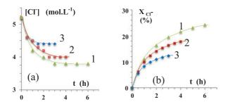
Fig. 3. Temporal evolution of both the concentration (a) of the chloride ion in the anolyte, and its conversion (b) in the outlet of the cathodic compartment, during galvanostatic electrolyses, for various feed solutions of brine ( $C_{NaCI} = 5$  M):  $Q_{NaCI}$  at 5 mol L<sup>-1</sup>: 60, 85, 135 cm<sup>3</sup>/h for curves 1 , 2 and 3 respectively. i = 1.7kA m<sup>-2</sup>;  $S_{anode}$  compartment = 150 cm<sup>3</sup>;  $S_{Cathode}$  Ti = 19 cm<sup>2</sup>;  $S_{$
