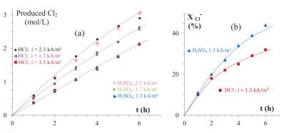
Fig. 7. Effect of both the acidic nature and the applied current density on the temporal evolution of: (a):  $Cl_2$  cumulated under NaOCI form in the 'gaseous  $Cl_2$  trapping solution (element 9, Fig. 2)'. (b):  $Cl_2$  conversion.  $Q_{acid}$  at  $G_{acid}$  at  $G_{acid}$
