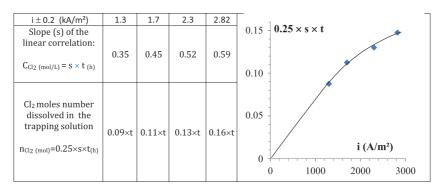
Fig. 5. Empirical correlations providing produced chlorine Cl<sub>2</sub> moles number dissolved in the trapping solution, as a function of both the electrolysis duration and the current density (results extracted from Fig. 4).
