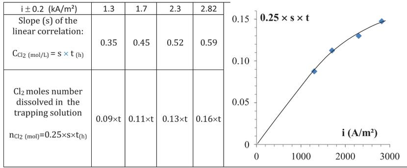
**Fig. 5.** Empirical correlations providing produced chlorine Cl<sub>2</sub> moles number dissolved in the trapping solution, as a function of both the electrolysis duration and the current density (results extracted from Fig. 4).
