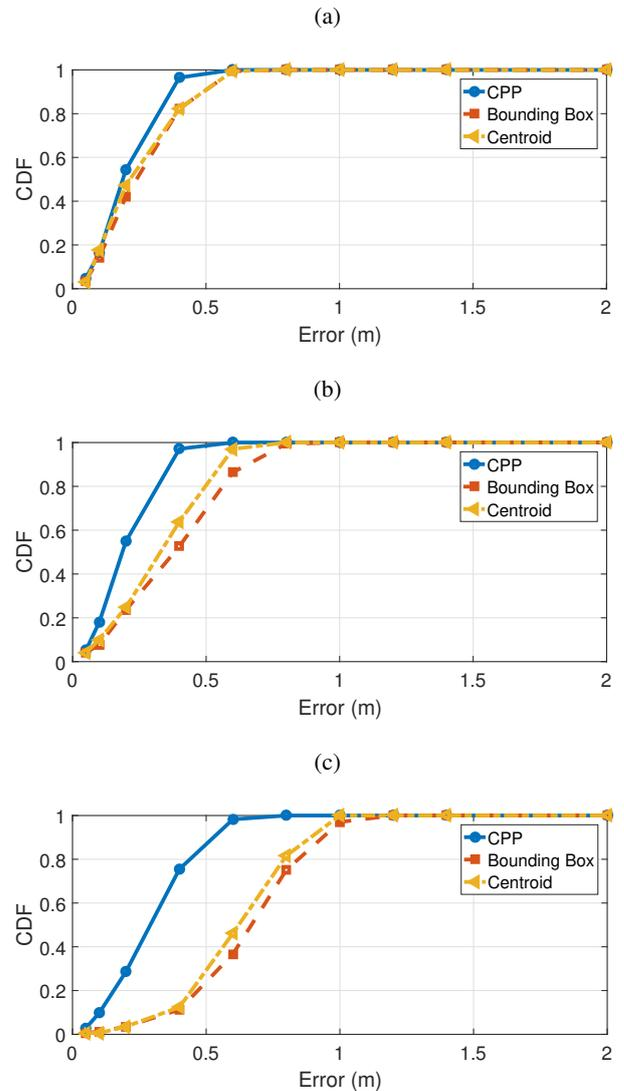
Fig. 8: Cumulative distribution function (CDF) for the proposed method, bounding box and centroid algorithm for (a)  $FOV=90^\circ$ , (b)  $FOV=110^\circ$  and (c)  $FOV=130^\circ$
