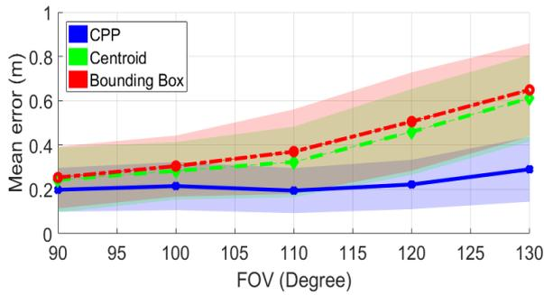
Fig. 7: Error performance and confidence interval of CP, Centroid and CPE for different FOV angles in the receiver side
