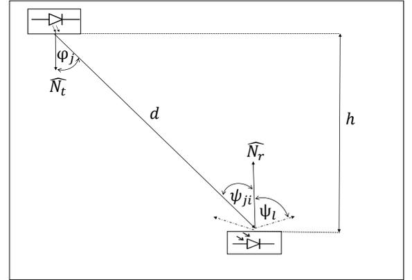
Fig. 2: VLC channel model
