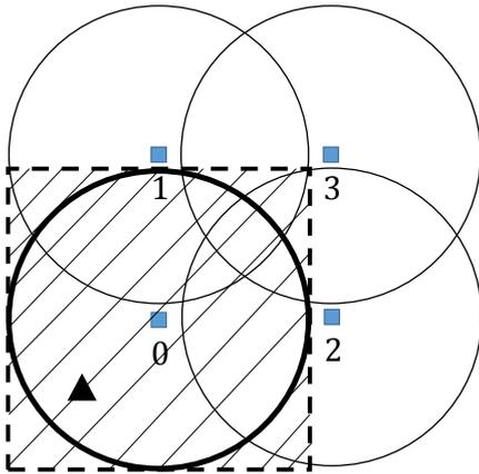
Fig. 4: Convex bounding box for the mobile node position
