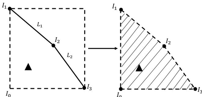
Fig. 6: Reduction of feasible localization area from bounding box rectangle to non-connectivity based polyhedron
