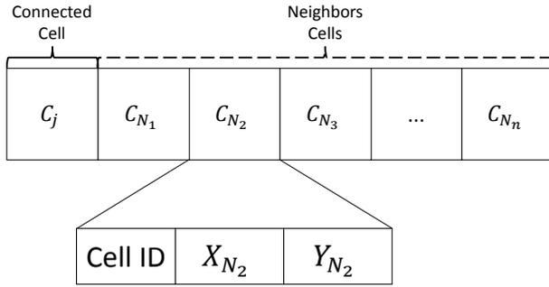
Fig. 3: Beacon transmitted by LED  $j$
