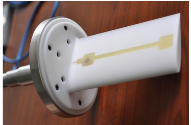
Figure 2. Cantilevered flexible hydrofoil equipped with strain gauges at the root
