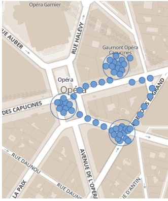
Fig. 3: Three POIs have been extracted from this mobility trace by using a clustering algorithm.
