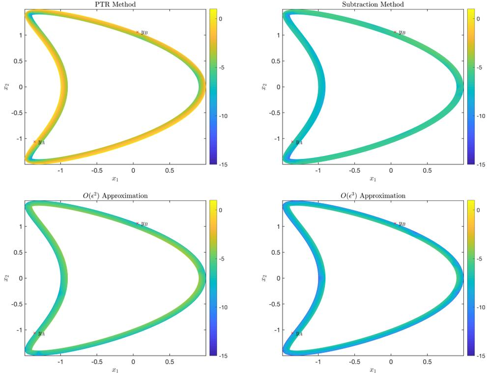
Figure 3: Plots of  $\log_{10}$  of the error for the evaluation of the double-layer potential in the kite domain defined by (6.2) using four methods: the PTR method (upper left), the subtraction method (upper right), the  $O(\varepsilon^2)$  asymptotic approximation method (lower left), and the  $O(\varepsilon^3)$  asymptotic approximation method (lower right). In each of these plots, boundary points  $y_A = (-1.3571, -1.0607)$  and  $y_B = (0.0571, 1.0607)$  are plotted as red  $\times$ 's.
