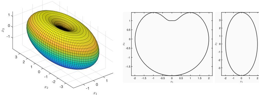
Figure 9: The boundary surface defined by (6.5) that is used to exemplify the evaluation of the double layer potential in three dimensions (left), and the intersections of this boundary with the  $x_1x_3$ -plane (center), and  $x_1x_2$ -plane (right).
