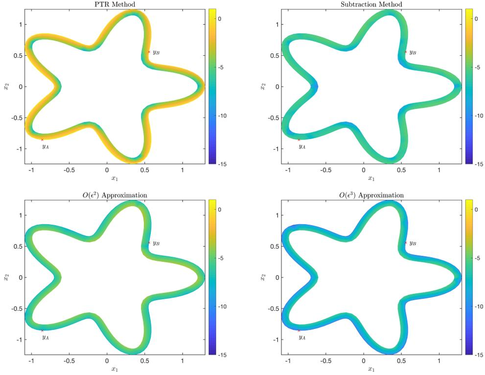
Figure 6: Plots of  $\log_{10}$  of the error for the evaluation of the double-layer potential in the star domain defined by (6.3) using four methods: the PTR method (upper left), the subtraction method (upper right), the  $O(\varepsilon^2)$  asymptotic approximation method (lower left), and the  $O(\varepsilon^3)$  asymptotic approximation method (lower right). In each of these plots, boundary points  $y_A = (-1.3571, -1.0607)$  and  $y_B = (0.0571, 1.0607)$  are plotted as red  $\times$ 's.
