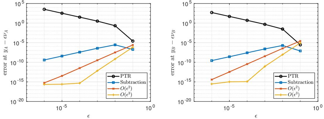
Figure 7: Log-log plots of the errors made in computing the double-layer potential by the four methods shown in Fig. 6 at  $y_A - \varepsilon\nu_A$  (left) and at  $y_B - \varepsilon\nu_B$  (right) for  $10^{-6} \leq \varepsilon \leq 10^{-1}$ .
