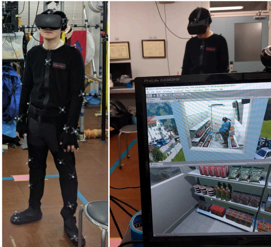
FIGURE 6 | Left: Participant in a motion capture suit. Right: A participant immersed in our virtual store in an obese virtual body. On the computer screen, the top view is a third person perspective view of the virtual environment while the bottom view corresponds to the participant's point of view.
