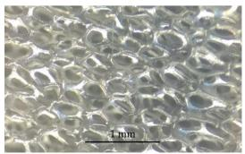
Fig. 3. Photography of the foam before lamination.
