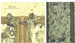
Fig. 14. Melted aluminium above the passivation protecting a gate finger (the dendrite of aluminium is roughly 25  $\mu$ m-high; left image) and below the piece of foam (right image).
