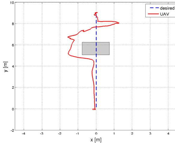
Fig. 9. Quadrotor surrounding an obstacle.
