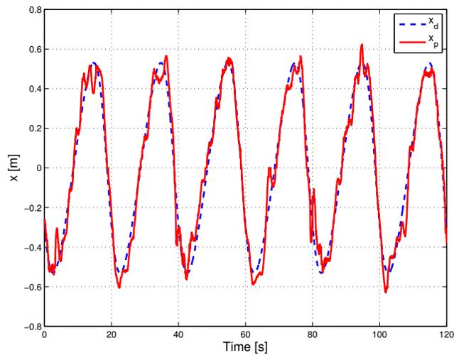
Fig. 4.  $x$  position response for a lemniscate trajectory.
