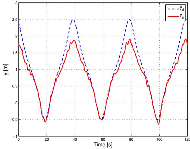
Fig. 5.  $y$  position response for a lemniscate trajectory.
