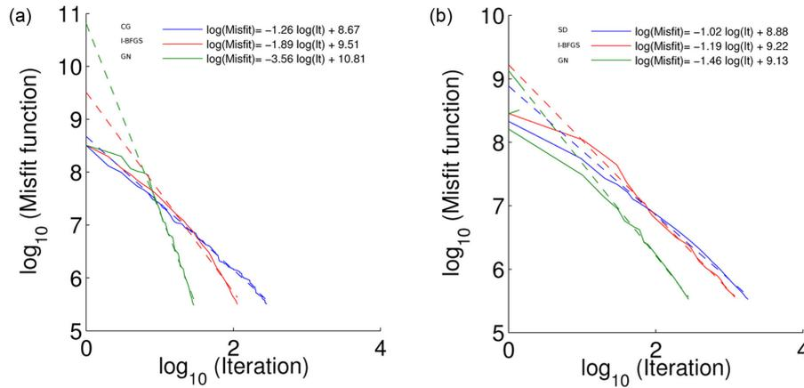
**Figure 3.** BP case study without noise: reduction of the misfit function as a function of the iteration on a log–log plot to extract the information on convergence rate. Blue: CG, Red: *l*-BFGS, green: GN. (a) Without source encoding. (b) With source encoding. The convergence rates of deterministic methods are higher than those of stochastic methods.
