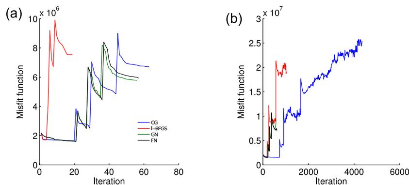
**Figure 9.** Valhall case study. Convergence of FWI. (a) Misfit function versus iteration number for the four frequency groups without SE. (b) Average over 50 independent realizations of the misfit function versus iteration number, for the four frequency groups with SE. Blue line:  $nl$ -CG optimization method. Red line:  $l$ -BFGS method. Green line: GN optimization method. Black line: FN optimization method.
