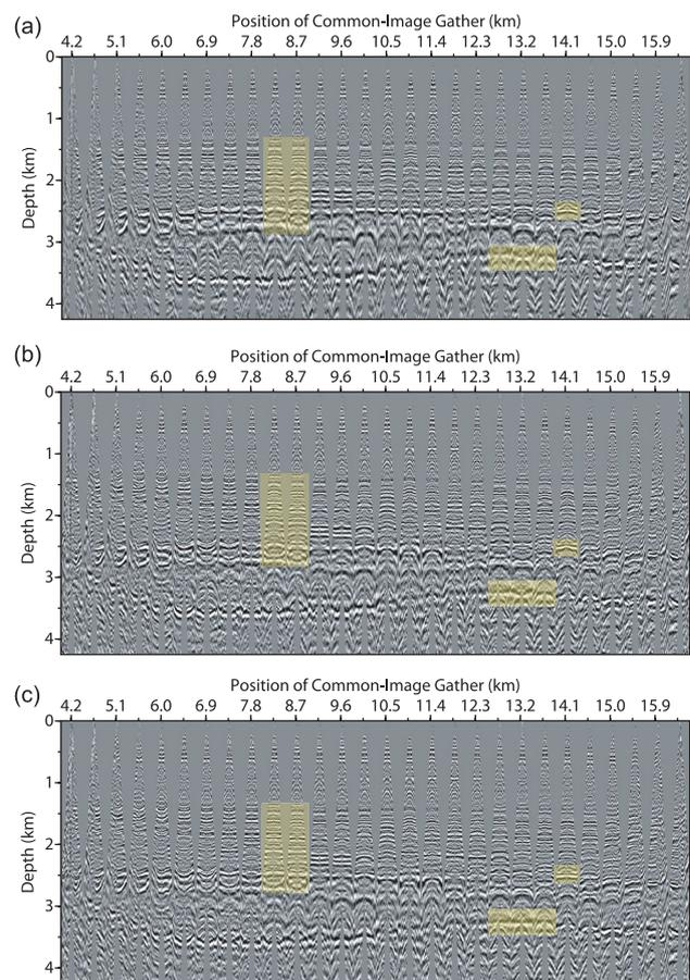
**Figure 16.** Valhall case study. Common image gathers in the offset-depth domain computed by reverse time migration performed in the initial model (a) and in the final FWI models inferred from the FN optimization method without (b) and with (c) source encoding. Reflectors which are flatter in the CIGs computed in the FWI model obtained with source encoding are highlighted.
