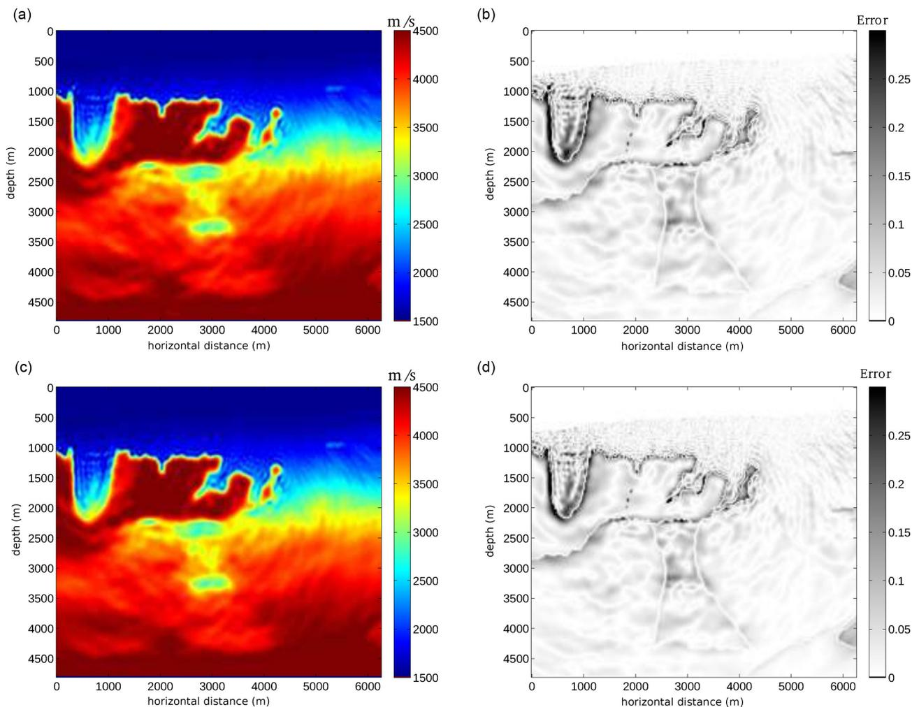
**Figure A2.** BP case study with noise. (a, c) Final FWI model for the GN optimization method used without (a) and with (c) source encoding ( $K = 3$ ). (b, d) Velocity model error (difference between the final FWI model and the true subsurface model).
