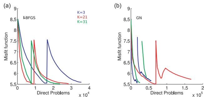
**Figure A8.** BP case study without noise. Average reduction of the misfit function versus number of forward problems with source encoding for different values of supersources  $K$ , over 50 realizations. Blue line:  $K = 3$ . Red line:  $K = 21$ . Green line:  $K = 31$ . (a) *l*-BFGS, (b) GN. There are originally 62 sources.
