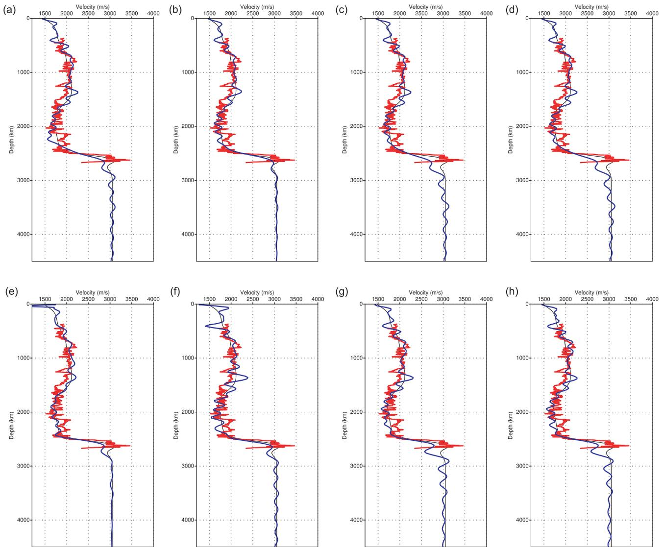
**Figure 11.** Valhall case study. (a–d) Logs of the final velocity models (blue lines) obtained without source encoding at a horizontal distance  $x = 9.5$  km for (e–h) Logs of the final velocity models (blue lines) when source encoding is used during FWI. (a, e) *nl*-CG/SD, (b, f) *l*-BFGS/BFGS<sub>s</sub>, (c, g) GN and (d, h) and FN. The sonic log is plotted with a red lines and the log of the initial model is plotted with a black line.
