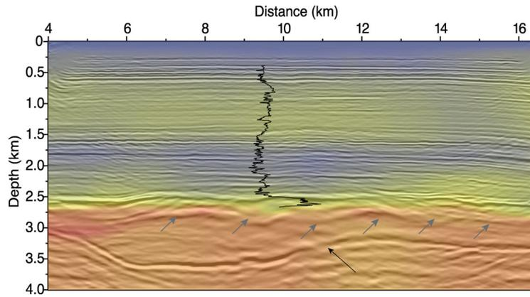
**Figure 8.** Valhall case study. Reverse time migrated image computed in the initial vertical velocity model, which is superimposed with a transparency. A sonic log located at 9.5 km in distance is also superimposed on the migrated image. The grey arrows delineate the base of the reservoir. The black arrow points a location in depth where the image of a deep reflector lacks continuity.
