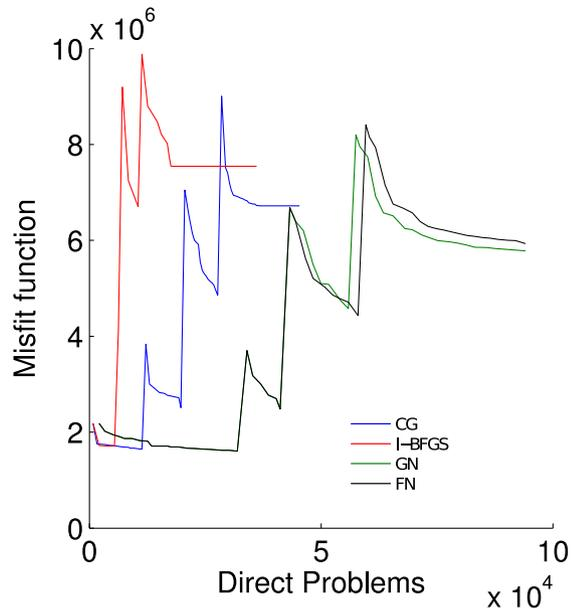
**Figure 12.** Valhall case study. Computational cost. Misfit function versus number of forward problems for each optimization method and for the four frequency groups when all the sources are processed independently. Blue lines: SD. Red lines: *l*-BFGS. Green lines: GN. Black lines: FN.
