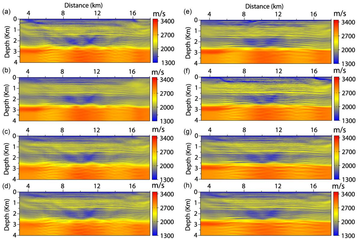
**Figure 10.** Valhall case study. Final FWI velocity models obtained without (a–d) and with (e–h) source encoding. (a, e)  $nl$ -CG/SD optimization method. (b, f)  $l$ -BFGS/BFGS<sub>r</sub> optimization method. (c, g) GN optimization method. (d, h) FN optimization method.
