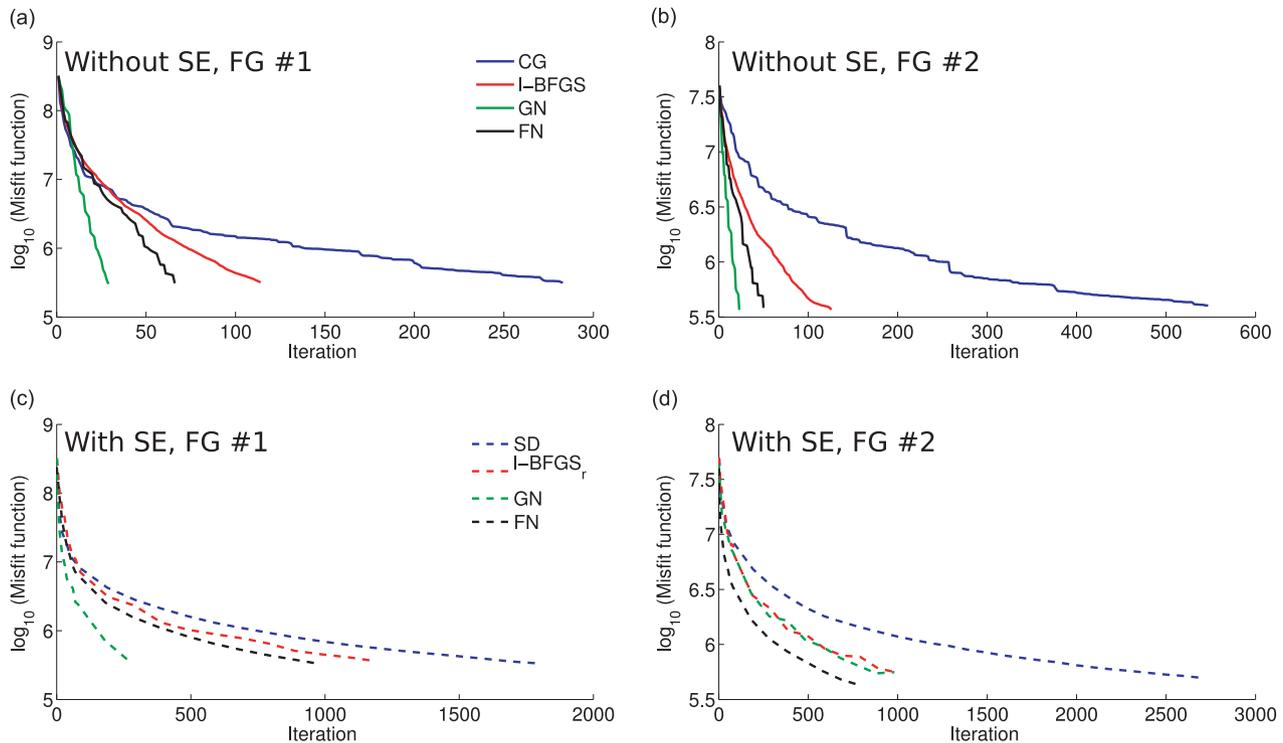
**Figure 4.** BP case study without noise: convergence rate. Reduction of the misfit function as a function of the iteration number without (a–b) and with (c–d) source encoding. (a, c) First frequency group (FG #1). (b, d) Second frequency group (FG #2). The curves are shown for the four optimization methods. Blue lines:  $n$  $l$ -CG/SD; red lines:  $l$ -BFGS<sub>r</sub>; green lines: GN; black lines: FN.
