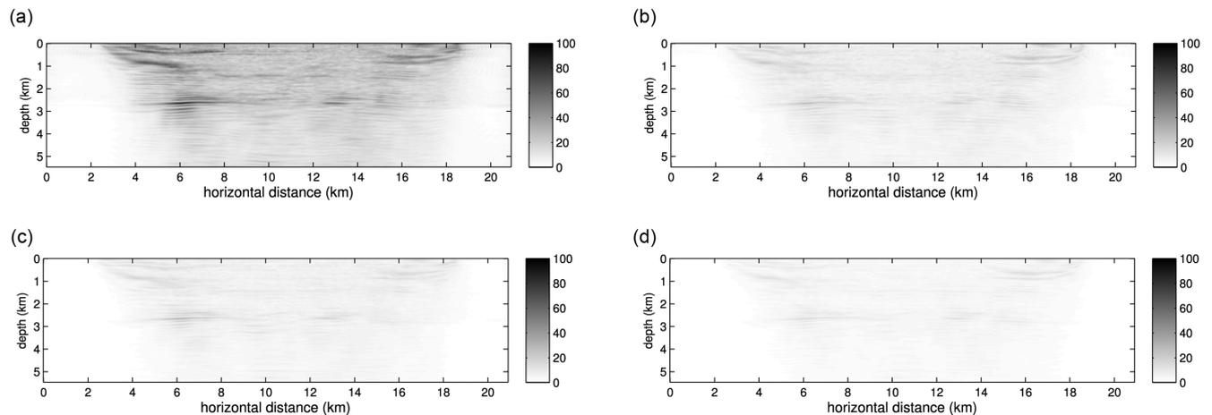
**Figure A12.** Valhall case study. Variance of the final velocity model (in  $\text{m s}^{-1}$ ) with source encoding using the Gauss-Newton optimization method for different values of supersources  $K$ . (a)  $K = 1$ , (b)  $K = 11$ , (c)  $K = 21$  and (d)  $K = 53$ .
