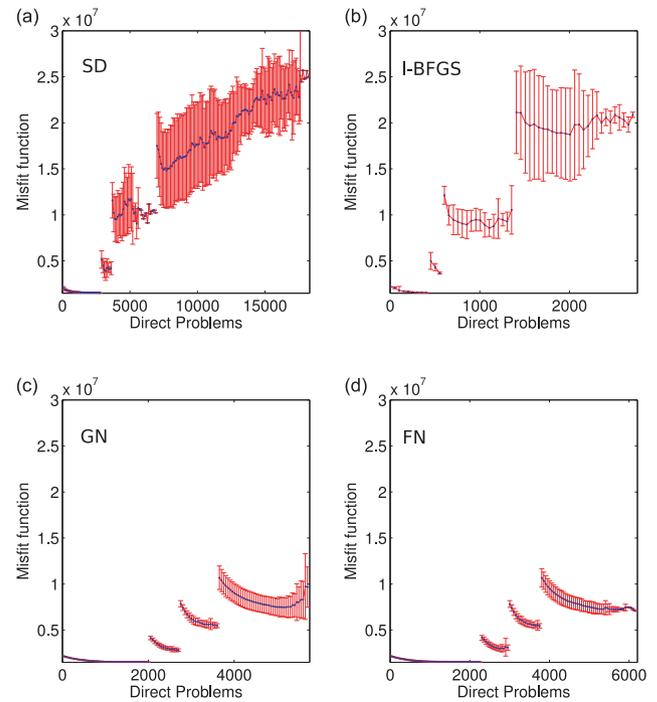
**Figure 13.** Valhall case study. FWI with source encoding. Mean value over 50 realizations of the reduction of the misfit function for the four frequency groups versus the number of direct problems. The variance of the misfit value is delimited with the red bars. (a) SD. (b) *l*-BFGS, (c) GN, (d) FN. Random variables follow a normal distribution.
