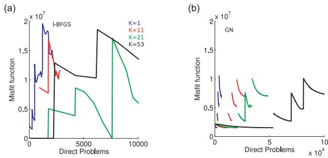
**Figure A10.** Valhall case study. Average reduction of the misfit function versus number of forward problems with source encoding for different values of supersources  $K$ , over 50 realizations. Blue line:  $K = 1$ . Red line:  $K = 11$ . Green line:  $K = 21$ . Black lines:  $K = 53$ . (a)  $l$ -BFGS, (b) GN. There are originally 210 sources.
