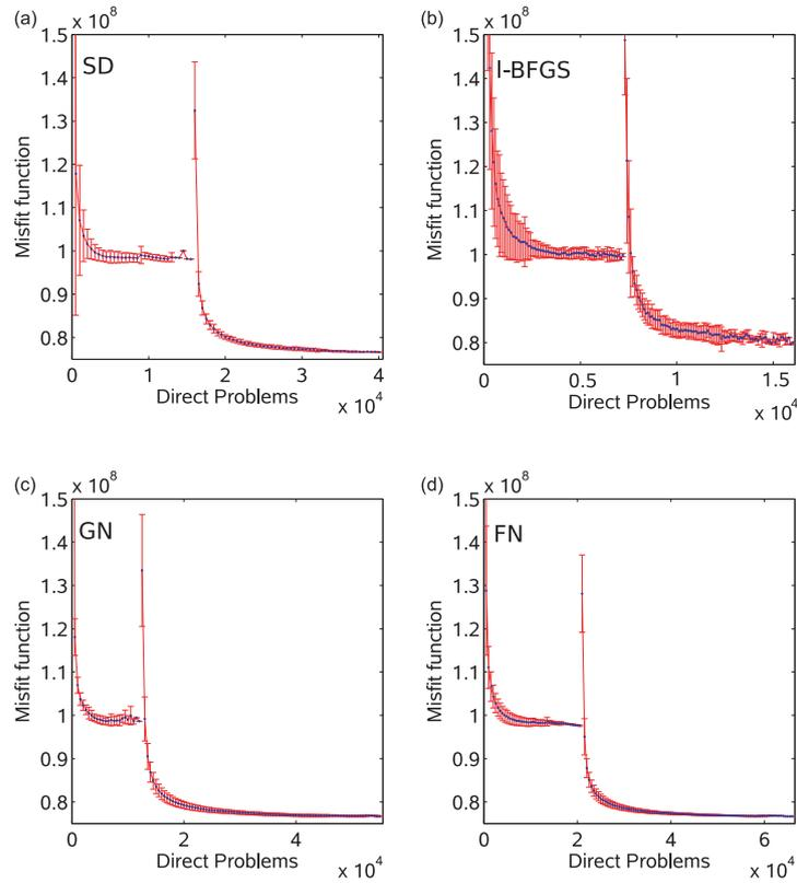
**Figure A4.** BP case study with noise. Mean value and variance of the misfit function value as a function of the number of forward problems for the first and second frequency group, during 50 independent realizations, using source encoding. (a) SD, (b) *l*-BFGS, (c) GN, (d) FN.
