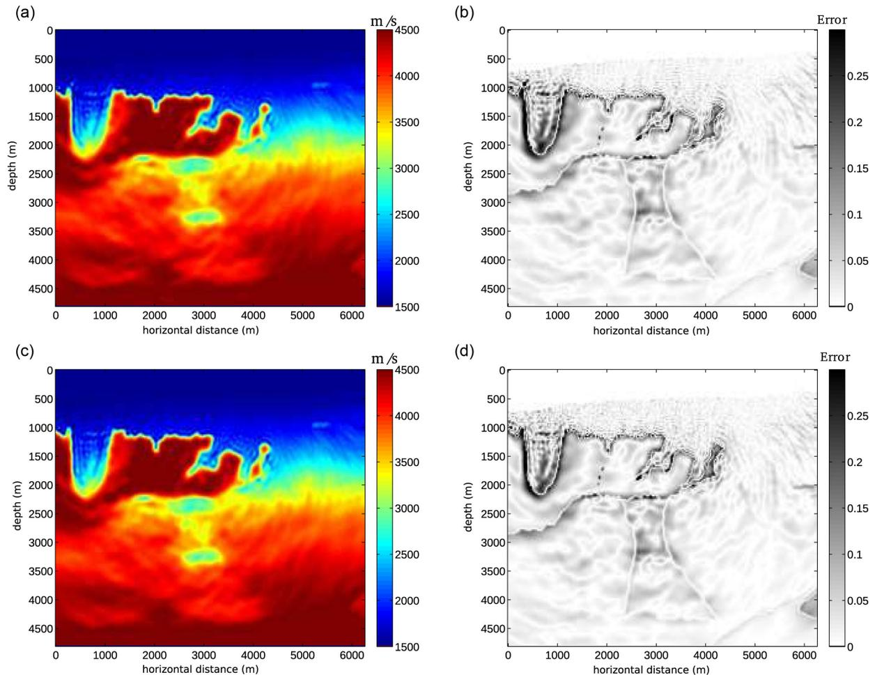
**Figure 5.** BP case study without noise. (a, c) Final FWI model for the GN optimization method without (a) and with (c) source encoding ( $K = 3$ ). (b, d) Velocity model error (difference between the final FWI model and the true subsurface model).
