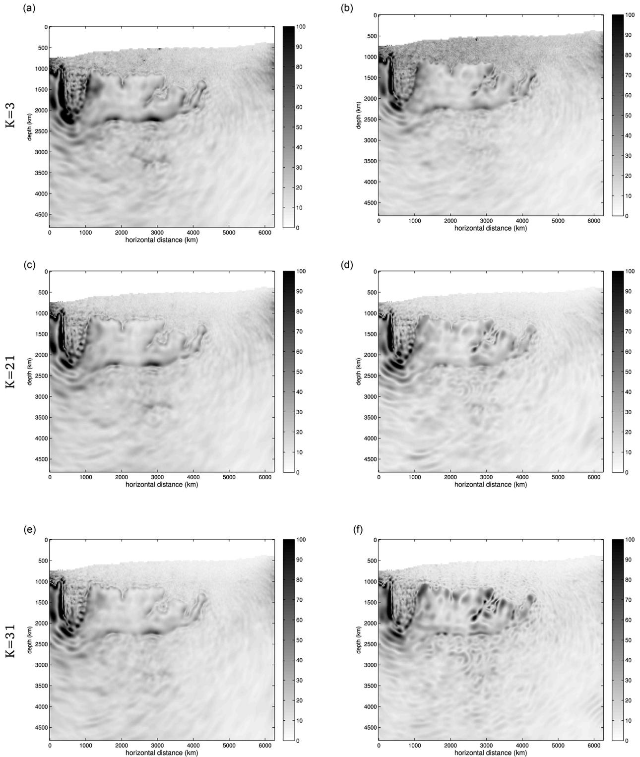
**Figure A9.** BP case study without noise. Variance of the final velocity model with source encoding for different values of supersources  $K$ , over 50 realizations. Panels (a), (c) and (e) correspond to an inversion with  $l$ -BFGS. Panels (b), (d) and (f) correspond to an inversion with GN. First row:  $K = 3$ . Second row:  $K = 21$ . Third row:  $K = 31$ . There are originally 62 sources.
