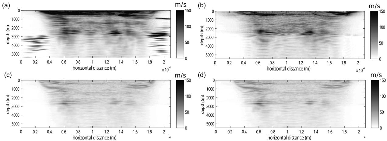
**Figure 14.** Valhall case study. Standard deviation of the final velocity model for 50 realizations of FWI with source encoding. (a) SD, (b)  $l$ -BFGS<sub>r</sub>, (c) GN, (d) FN. Random variables follow a normal distribution.
