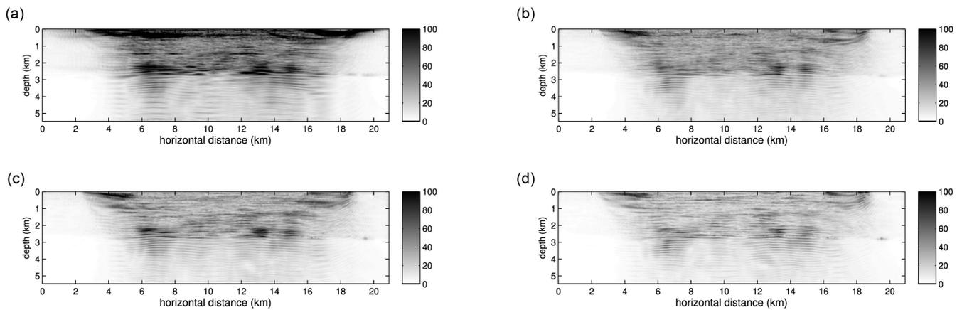
**Figure A11.** Valhall case study. Variance of the final velocity model (in  $\text{m s}^{-1}$ ) with source encoding using the  $l$ -BFGS optimization method for different values of supersources  $K$ . (a)  $K = 1$ , (b)  $K = 11$ , (c)  $K = 21$  and (d)  $K = 53$ .
