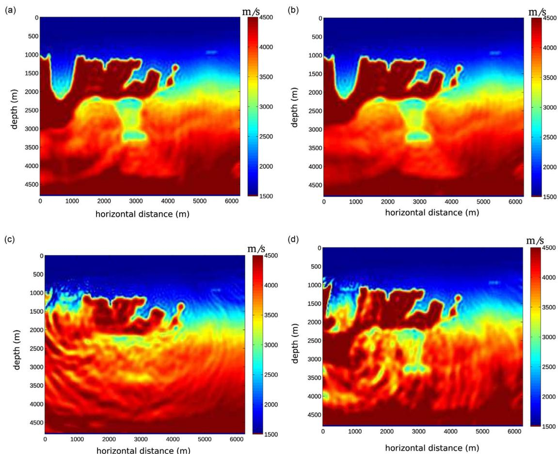
**Figure A6.** BP case study without noise. (a and b) Final velocity models obtained by inverting a single frequency group containing nine frequencies between 1 and 9 Hz without (a) and with source encoding (b) and with the initial velocity model shown in Fig. 1(b). (c and d) Same as (a and b) with the smoother initial velocity model shown in Fig. 1(c). Note how source encoding allows to reach an improved local minimum.
