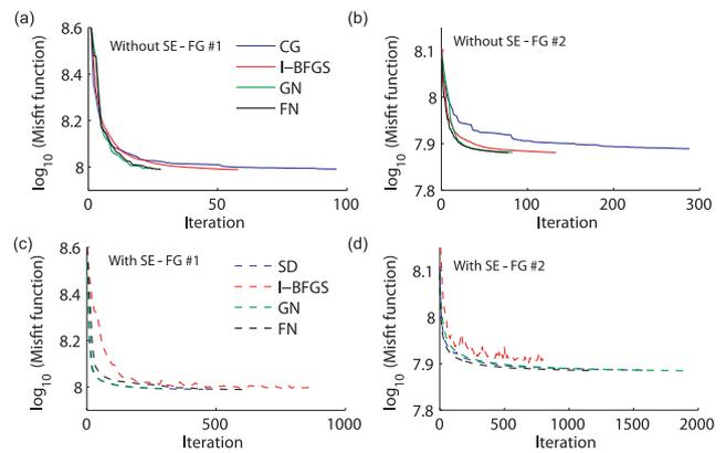
**Figure A1.** BP case study with noise: convergence rate. Reduction of the misfit function as a function of the iteration number without (a–b) and with (c–d) source encoding. (a, c) First frequency group (FG #1). (b, d) Second frequency group (FG #2). The curves are shown for the four optimization methods. Blue lines: *nl*-CG; red lines: *l*-BFGS; green lines: GN; black lines: FN.
