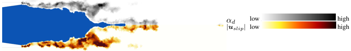
Figure 5: NIR7eq with atomization (Legend: blue isovolume of \alpha_2 = 0.99 , volume fraction of droplets in the SPIREE solver \alpha_d , slip velocity norm |\mathbf{u}_{slip}| )
