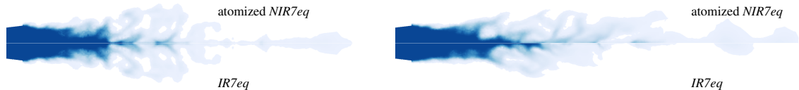
Figure 6: Comparison of the liquid volume fraction \alpha_2 : slice at \theta=\pi/6 , at \tau=\tau_1 (left) and \tau=\tau_1+1.5\tau_{conv} (right), \alpha_2=1.0 \rightarrow \alpha_2=0.01
