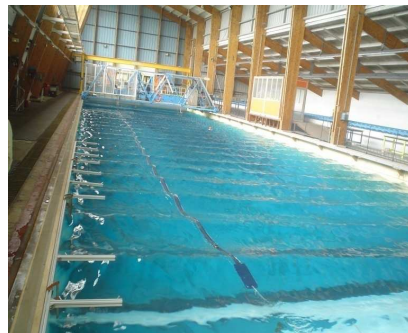
Fig. 10 Optical fiber laying on the water surface
