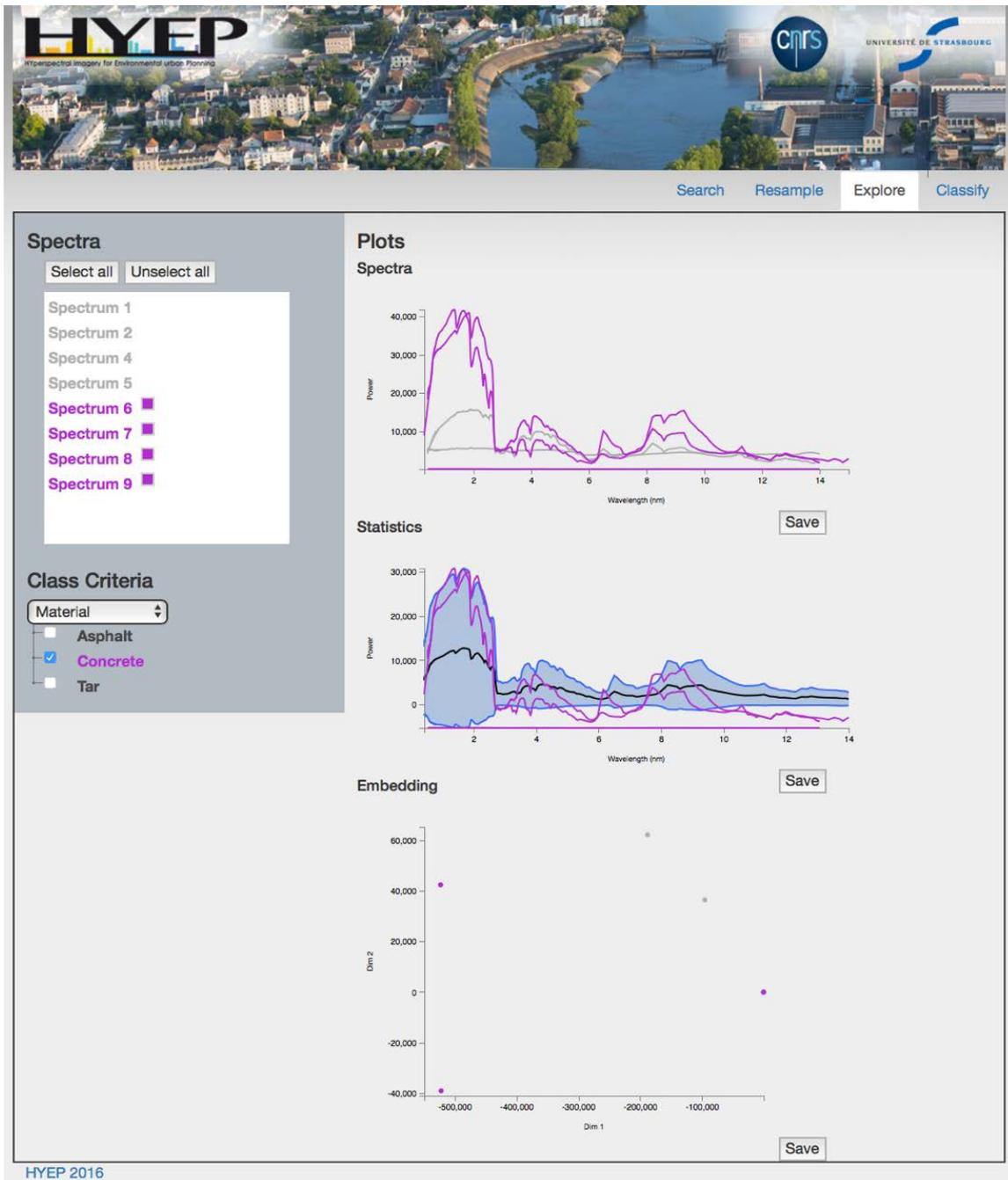
Figure 4: The Explore page, displaying the functionality of selecting a specific criterion to highlight all the spectra that belong to that criterion (Material, CLC classification, Sensor, Data Source, etc.).
