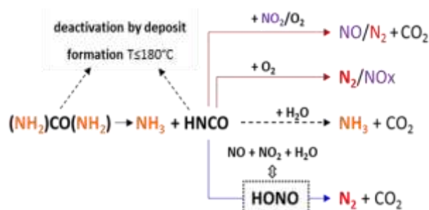
Scheme 1. Proposal of HNCO competitive reactivity for Urea-SCR with shortened urea residence time.
