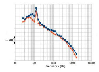
**Figure 3.** Sound pressure level at the chimney outlet [dB] – 900 RPM (red) – 1000 RPM (blue)
