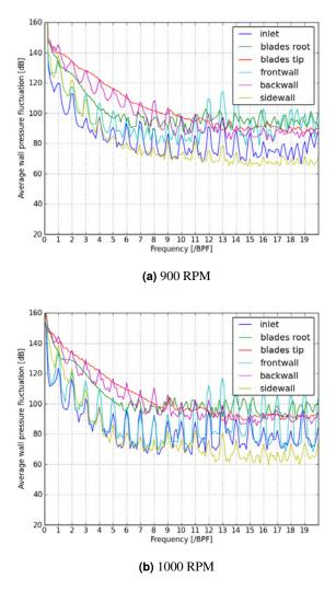
**Figure 12.** Maximum amplitudes of wall pressure fluctuations.
