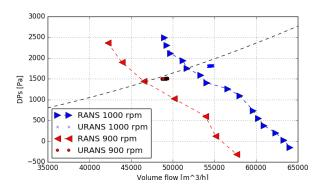
Figure 5. Performance curves – 900 RPM and 1000 RPM
