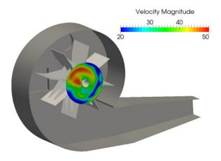
Figure 8. Inlet flow distorsion – 1000 RPM URANS.
