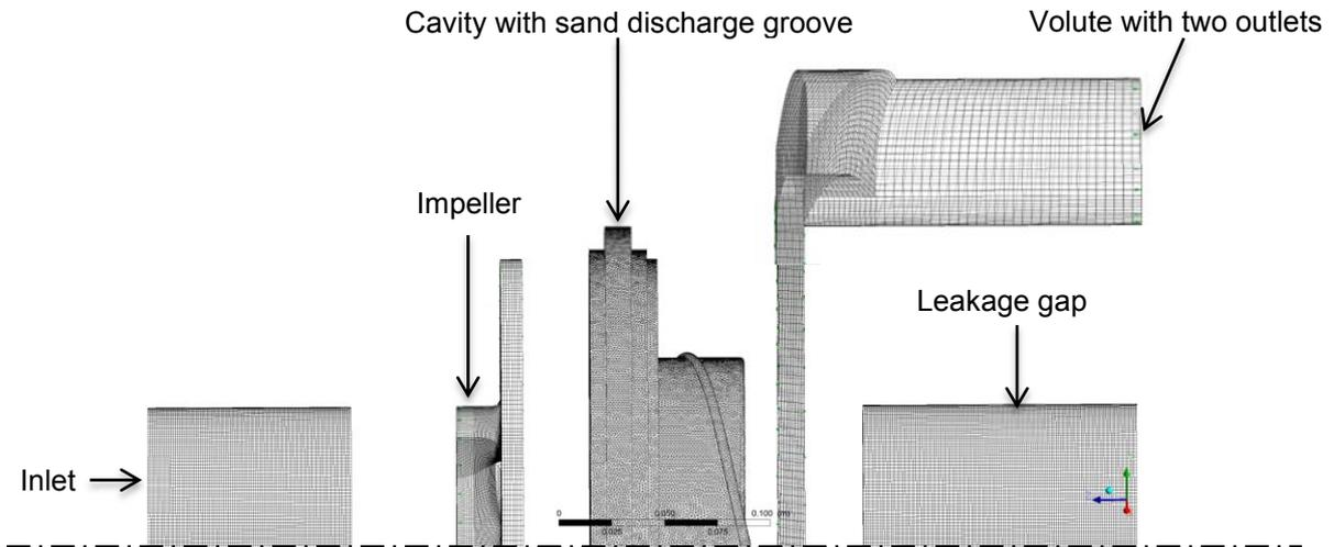
Figure 3. Domains and Meshes of Simulation Model
