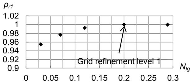
Figure 5: Mesh Sensitivity Analysis
