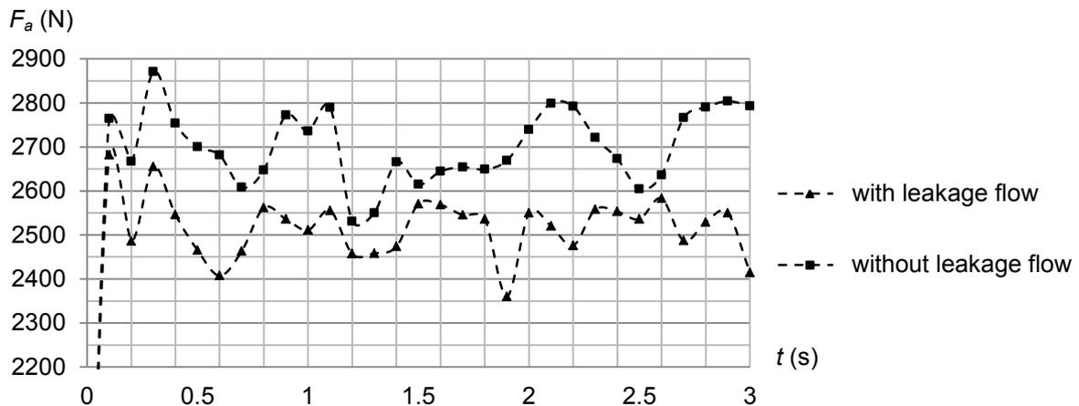
Figure 13. Variations of the Axial Thrust of the Last Stage
