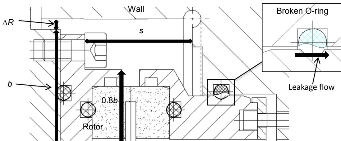
Figure 2. Sand Discharge Groove in the Rear Chamber and Leakage Flow
