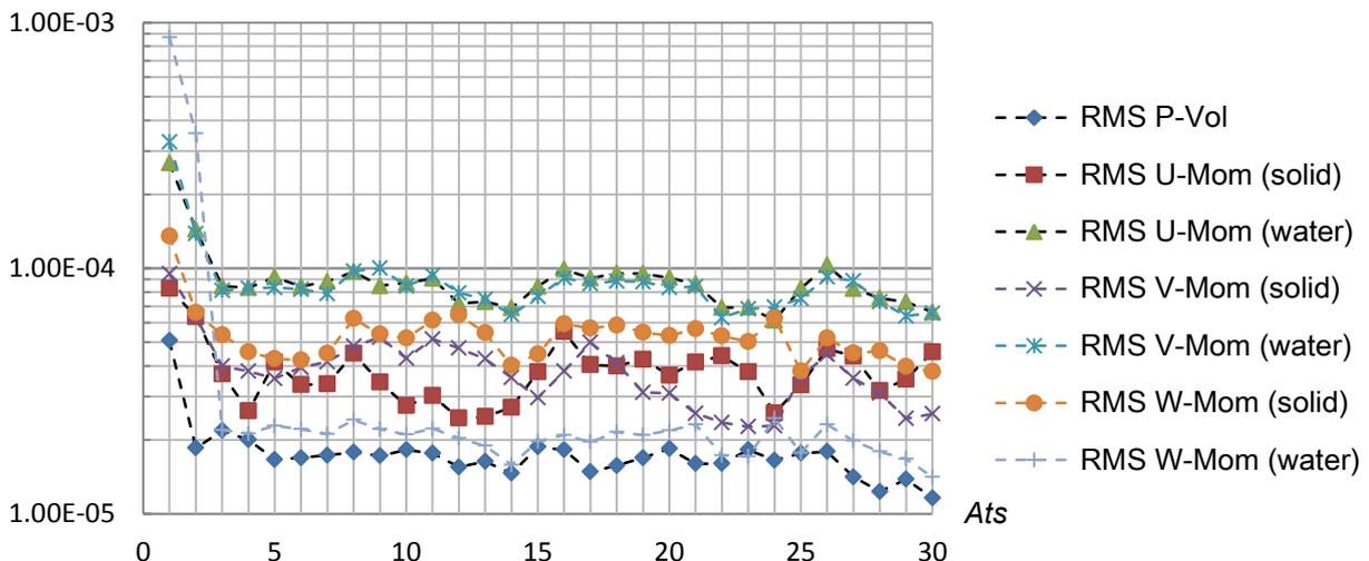
Figure 6. Convergence Behavior of Simulation with Leakage Flow
