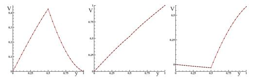
**FIGURE 3.** Study of the fluid-structure interaction between a viscous fluid and an elastic solid with a periodic evolution. The viscosity of the fluid is equal to  $\nu = 1$  and the solid shear modulus is equal to  $\nu = 4$ . Velocity profile based on y for times t = 10 s, t = 10.5 s, t = 10.8 s are plotted. In solid lines the theoretical solution is reported. The dots correspond to a spatial approximation of a 32 mesh for  $y \in [0, 1]$ .
