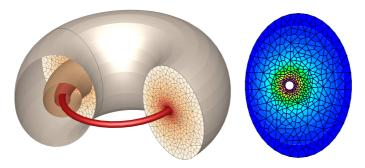
**FIGURE 4.** Magnetic field created by a circular turn crossed by a current I within a torus of elliptical section. The unstructured mesh is composed of non-regular hexahedra [19]. On the left is the torus coil surrounded by isovalues of the magnetic field and on the right, a cross-section representing the potential field is shown.
