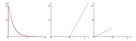
**FIGURE 2.** Fluid-structure interaction between a viscous fluid and an elastic solid; the viscosity of the fluid is equal to  $\nu = 1$  and the solid shear modulus is equal to  $\nu = 4$ . On the left, the velocity of the interface over time is presented, in the center, the velocity **V** at steady-state regime is reported and on the right, the displacement of the solid **U** plotted.
