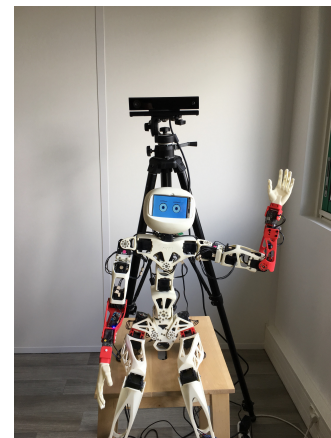
Fig. 1: Setting of the system including a Microsoft Kinect v2 and an open source humanoid robot called Poppy.
