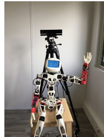
Fig. 1: Setting of the system including a Microsoft Kinect v2 and an open source humanoid robot called Poppy.
