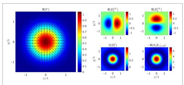
**Figure 1.** A real-valued Gaussian potential  $V \propto \exp(-2r_{\perp}^2/\lambda^2)$  produces a radially polarized beam. The transverse electric field  $E_{\perp}^{f,V}$  is indicated by arrows. The induced field components and the 'charge density'  $-\partial_z E_z|_{z=0}$  are shown on the right.
