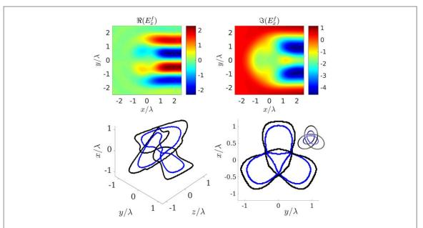
**Figure 8.** Two linked trefoils in different components of the electric field: the blue line represents the vortex line in  $E_y$ , the black line the vortex line in  $E_z$ . The corresponding (semi-infinite) profiles in  $E_x^f$  are shown in the upper panels.
