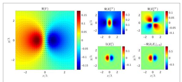
**Figure 4.** A real-valued dipole is prescribed in  $\partial_z E_z|_{z=0}$ , and the resulting potential  $V=\phi^{\text{dipole}}$  (see text for details) is used to compute the electric field components.
