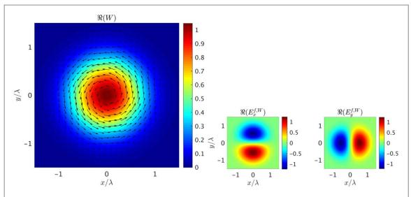
**Figure 2.** A real-valued Gaussian potential  $W \propto \exp(-2r_{\perp}^2/\lambda^2)$  produces an azimuthally polarized beam. The purely transverse electric field  $E_{\tau}^{f,W}$  is indicated by arrows. The induced field components are shown on the right  $(E_{\tau}^{f}=0)$ .
