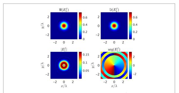
**Figure 6.** A bell-shaped circularly polarized transverse field produces a singly charged vortex in  $E_z^f$ . The off-axis sign flips in the phase plot are due to the filter function  $H_{k_0}$  (see text).
