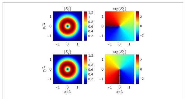
**Figure 3.** Transverse field components of a circularly polarized single charge vortex beam produced by complex superposition of figures 1 and 2, that is,  $V = iW \propto \exp(-2r_{\perp}^2/\lambda^2)$ .
