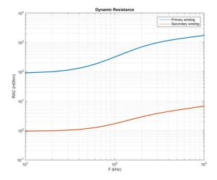
Fig. 10. Analytical winding AC resistances
