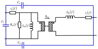
Fig. 7. High frequency equivalent circuit of a planar transformer
