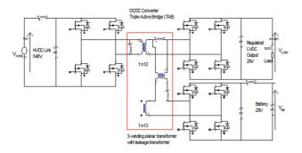
Fig. 3. TAB simplified electric diagram
