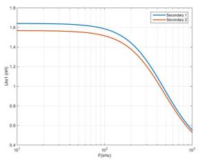
Fig. 12. Analytical leakage inductances from secondary windings
