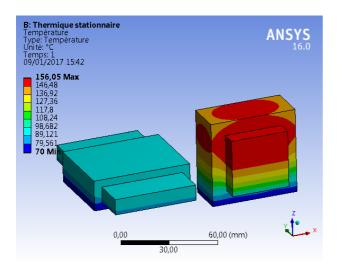
Fig. 11. Temperature distribution in planar vs conventional transformer
