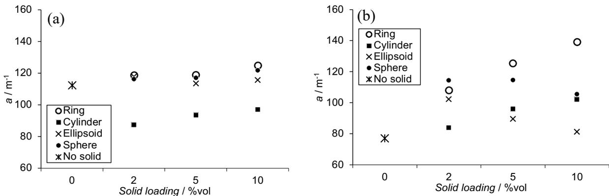
**Figure 6** Effect of the solid particles on the specific interfacial area at superficial velocity of  $1.3 \times 10^2$  m/s using (a) small orifice sparger (b) large orifice sparger
