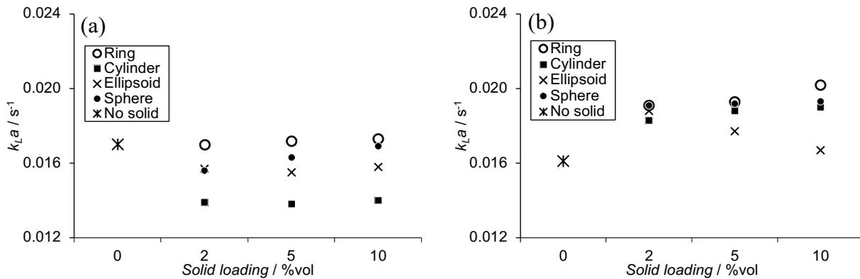
**Figure 7** Effect of the solid particles on the overall volumetric mass transfer coefficient at superficial velocity  $1.3 \times 10^{-2}$  m/s using (a) small orifice sparger (b) large orifice sparger
