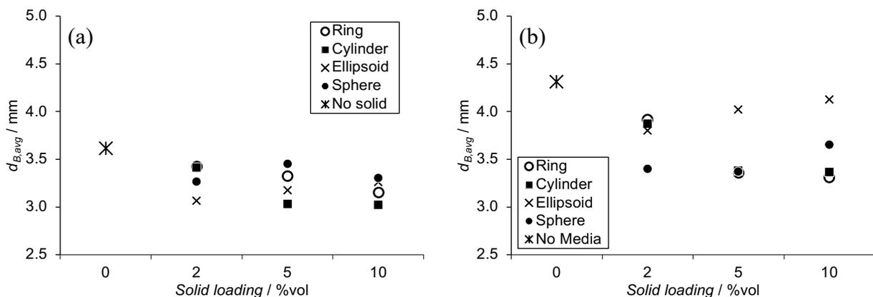
**Figure 3** Effect of the solid PP particles on the average bubble diameter at superficial velocity of  $1.3 \times 10^{-2}$  m/s using (a) small orifice sparger and (b) large orifice sparger
