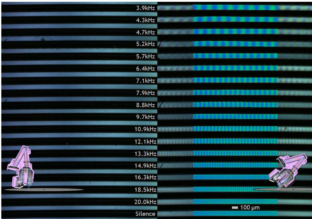
Fig. 6. A composite of 2x5 pictures from AES 78rpm coarse groove 2007 test disc shown in Figure 2, inner and densest sweep track; signal is accessible on the whole height span of the groove wall, up to 20kHz. Left: viewed from top, tracks are dark and highest frequencies are indistinguishable from silence. Right: scanned at 45° degrees; tracks are blue-green. For a better visibility, saturation and luminance are normalised in the exploited central area.
