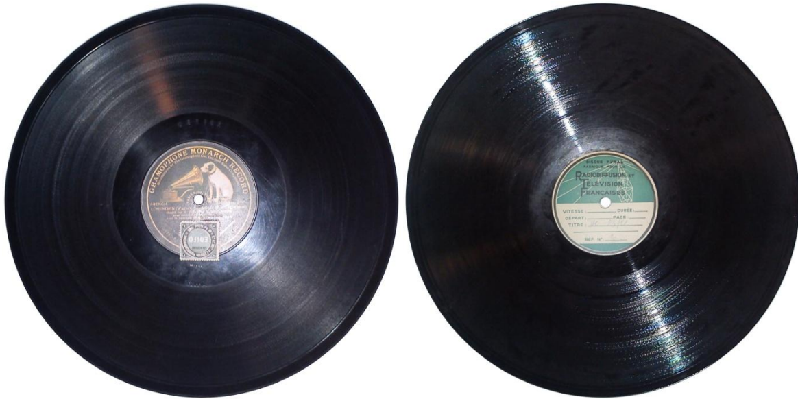
Fig. 1. Left: a printed “shellac” disc (~1920); right: a one-off lacquer “direct recording” disc (1951)
