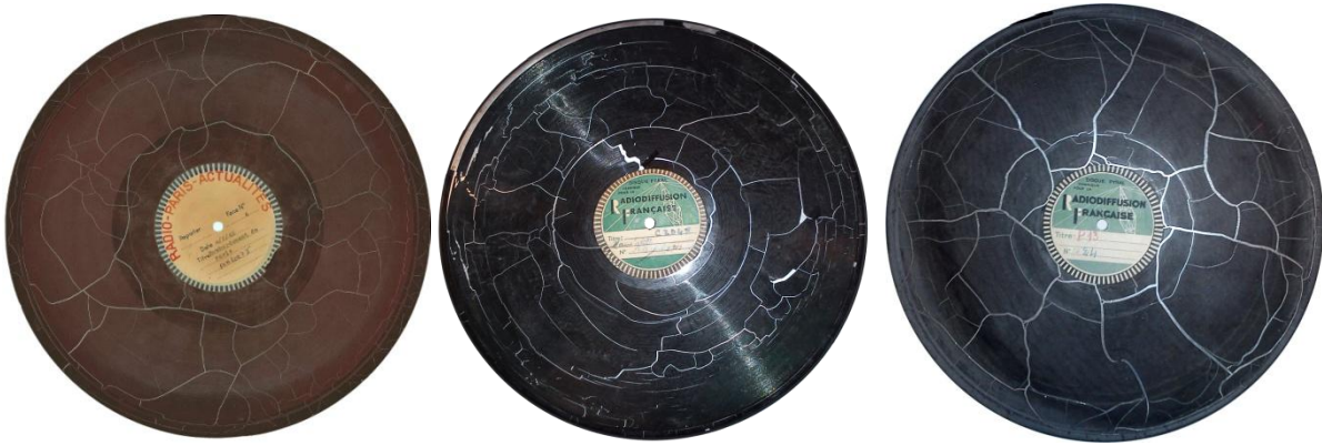
Fig. 14. Examples of cracked lacquer discs
