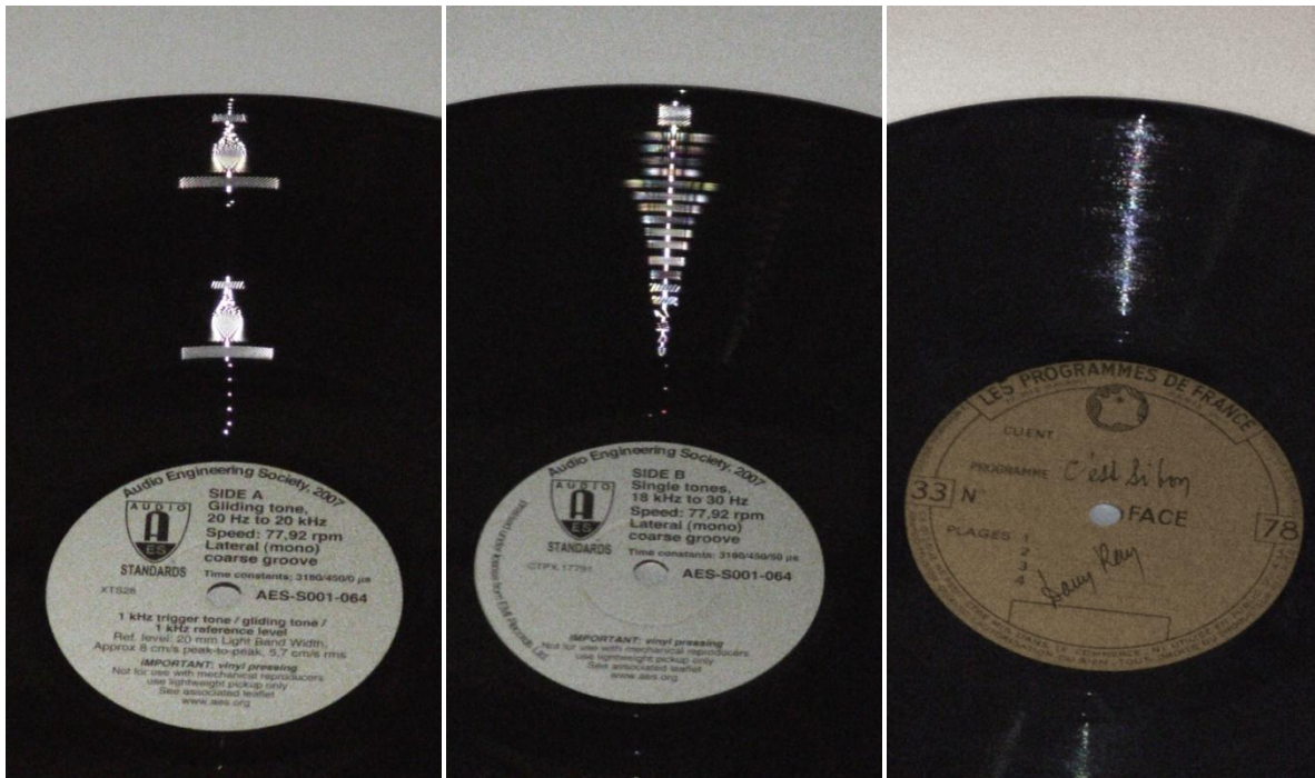
Fig. 2. The Buchmann-Meyer method was an easy way of measuring the peak radial cutter velocity, by measuring the width of the reflected pattern from a collimated light source, up to the point the maximum velocity was often expressed in mm Light Band Width (LBW). Left and center: AES coarse-groove 2007; right: a direct-cut lacquer recording.
