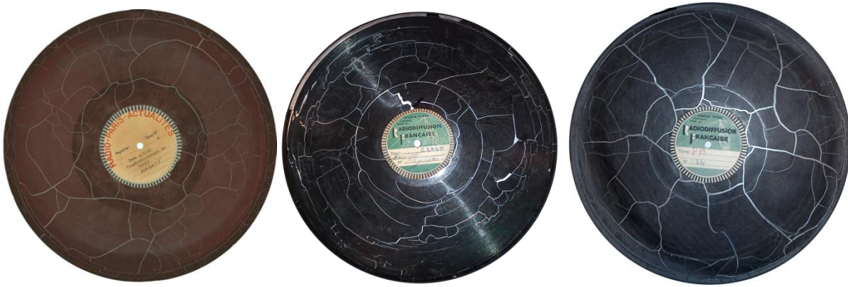
Fig. 14. Examples of cracked lacquer discs
