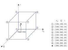
Fig. 14: The "target" material (black dot) and eight different parameter combinations chosen as initial points in parameter space.
