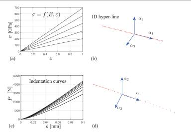
Fig. 4: An illustrative example of MDS applied to Hooke's law: (a)-(c) Stress-strain curves; and (b)-(d) indentation curves for sampled elastic materials.
