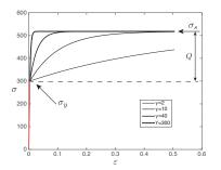
Fig. 2: Voce law with three hardening parameters:  $\sigma_y$ , Q and  $\gamma$ .
