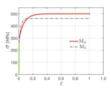
Fig. 11: A comparison of tensile curves for (M<sub>4</sub>, M<sub>5</sub>) rebuilt using Voce law with the identified parameters.
