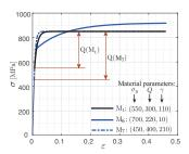
Fig. 17: Two mystical material pairs using the Voce hardening law: (M<sub>t</sub>, M<sub>6</sub>) the *true* mystical material pair, and (M<sub>t</sub>, M<sub>7</sub>) the *false* mystical material pair.
