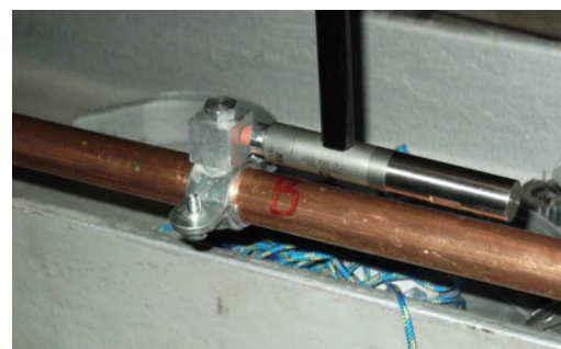
Figure 5. Modal hammer with elastic tip used for generating pipeline transient vibrations
