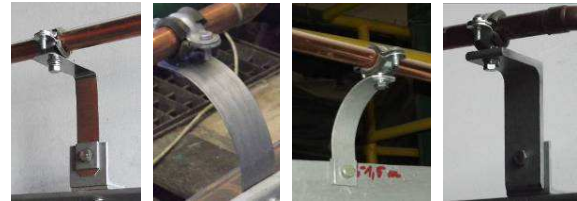
Figure 4. Flat springs (from the left) FS2, FS3, FS4, and FSR for supporting the pipeline
