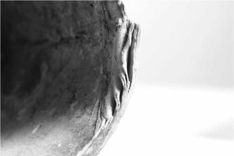
FIGURE 16. (a) Close-up image of mouth and labium of one of the smallest pipes. (b) close-up image of the edge of a pipe, showing the degradation and the partial detachment of the paper layers.
