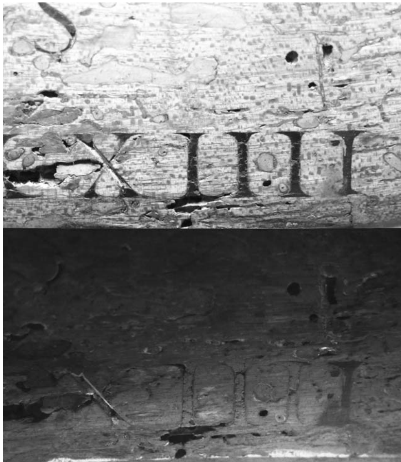
FIGURE 14. Visible light and UV image of the date, inlaid on the front panel above the keyboard. The different fluorescence of the last letter is clearly visible. Photo by Jean-Philippe Echard, © Cité de la Musique. See color photo p. 201.
