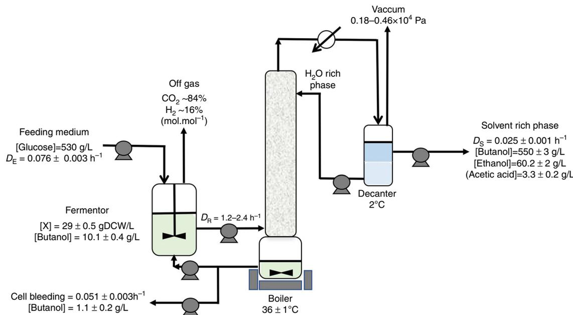
**Fig. 4** Schematic representation of the extractive continuous fermentation process. The fermentor, boiler, and decanter have working volumes of 0.5 L, 0.3 L, and 0.1 L, respectively. For more details see Methods
