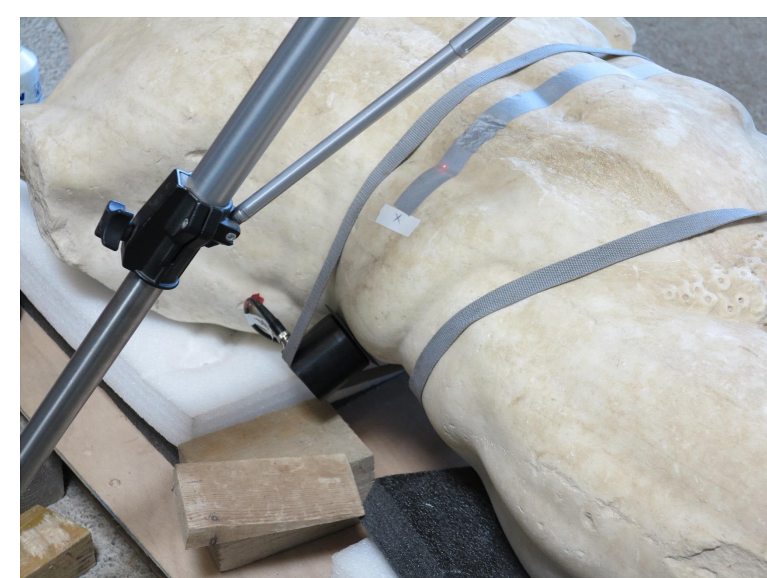
Auscultation of the marble homogeneity at the level of the hip
