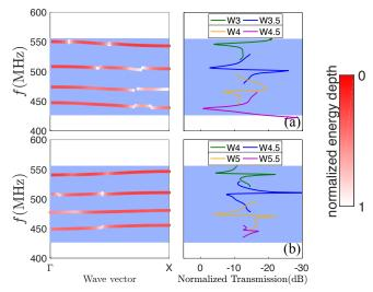
FIG. 9: Normalized transmission spectra for the defectincluded PnC on the (a)  $5^{th}$  and (b)  $6^{th}$  cavity mode. Corresponding dispersion curve for each peak is shown on the left. Blue zones denote the predicted band gap of the perfect PnC. r = 0.2a, H = 0.6a,  $a = 4\mu$ m,  $N_{PnC} = 4$ .
