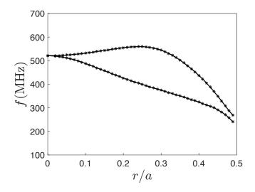
FIG. 3: Love modes eigenfrequencies of the PnC as a function of the hole radius. Between the two black curves representing the two Love modes is the band-gap region of the PnC. H = 0.6a,  $a = 4\mu$ m.
