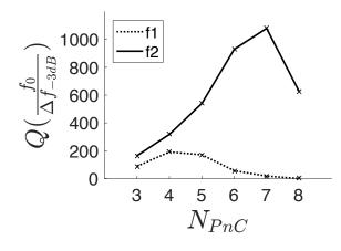
FIG. 11: Quality factors of the defect modes as a function of the number of PnC holes on each side of the cavity.  $W = 5a, r = 0.2a, H = 0.6a, a = 4\mu m.$
