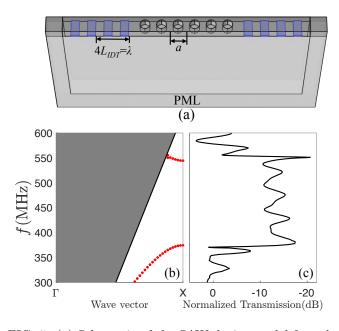
FIG. 5: (a) Schematic of the SAW device model for calculating the transmission spectra of Love waves through the PnC. r = 0.3a, H = 0.6a,  $a = 4\mu$ m; (b) Zoom of the band structure of Love modes around the band-gap zone in the  $\Gamma$ -X direction; (c) Normalized transmission spectra of Love waves propagating through the PnC around the band-gap zone.  $N_{PnC} = 10$ ,  $N_{IDT} = 20$ ,  $h_{IDT} = 200$ nm,  $V_0 = 1V$ .
