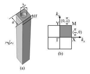
FIG. 1: (a) Unit cell of the PnC with cylindrical holes arranged in square array in the silica film. The substrate is 90ST-cut quartz. r = 0.3a, H = 0.6a,  $a = 4\mu$ m; (b)  $1^{st}$  BZ of the PnC. The gray square is the irreducible BZ;
