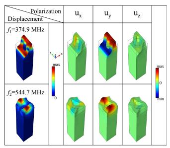
FIG. 4: Displacement fields and polarizations of the two Love modes at 374.9 and 544.7 MHz. r = 0.3a, H = 0.6a,  $a = 4\mu$ m.
