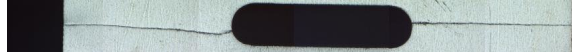
FIG. 2: Photography of the specimen with a crack perpendicular to fiber direction - With permission of ONERA/DMAS, Châtillon, France
