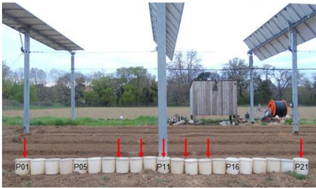
Figure 1. Effective rain and soil water content measurement under solar panels. Red arrows indicate the position of neutron probes, on a line parallel to that of the collectors, 1 m before it. Some of the P01 to P21 collectors have been identified on the picture for clarity.
