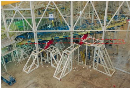
FIGURE – Test torsion aile A380 (supaero)
