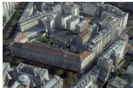
Figure 2. 3D model of a detail of the 12th district of Paris, GSD 15cm [Courtesy: Laboratoire MATIS, IGN France]
