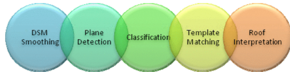
Figure 3. Sequence of the five major processing steps
