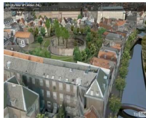
Figure 1. 3D city model, LOD2 (detail of Leiden, Netherlands) [Courtesy: Aerodata International Surveys, Belgium, http://www.aerodata-surveys.com/ ].
