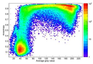
**Fig. 2**. Histogram of the degree of anisotropy versus average grey value computed from the real UC model with 10-pixel voxel size.
