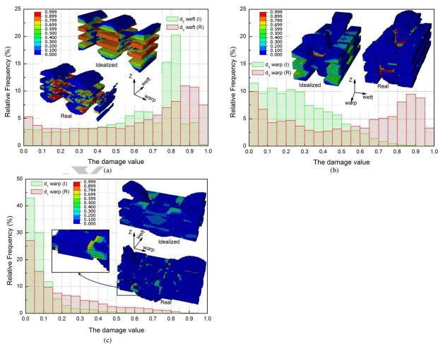
Fig. 14. The statistical distribution of the damage value at the time when peak stress value is reached: (a) transverse matrix crack in wefts  $(d_2)$ ; (b) delamination of yarn in collective warps  $(d_3)$  and (c) yarn breakage in the warps  $(d_1)$ .
