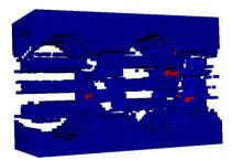
(a) damage initiation at tensile strain 0.27%
