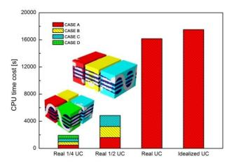
Fig. 11. CPU time cost versus homogenization strategies.
