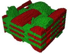
Fig. 4. The real voxel UC model (with the matrix hidden), created from the CT image.
