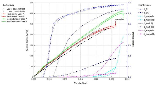
Fig. 12. Simulated stress-strain curves along with the experimental upper and lower bounds (Left-y-axis); evolution history of d<sub>i</sub> in matrix/collective warps/wefts component (Right-y-axis).
