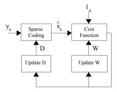
Fig. 1. A signal  $y_k$  associated to a label  $l_k$  is encoded by a dictionary D, the resulting code  $\hat{x}_k$  is used as an input to a cost function with parameters W. The cost function  $\mathcal{L}(l_k, \hat{x}_k, W)$  is computed. Then, the dictionary D and the parameters W are updated to fit the classification problem.
