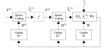
Fig. 3. Structure with 2 layers. Input vectors  $\mathbf{Y}^{(1)}$  go through a sparse coding step. We have  $\mathbf{Y}^{(2)} = f(\hat{\mathbf{X}}^{(1)})$  as input to the second layer.  $l_k$  is the label of the image and the function f models pulling and concatenation operations. Back-propagation is then used to update both dictionaries  $D^{(1)}$ ,  $D^{(2)}$  and the parameters W simultaneously.
