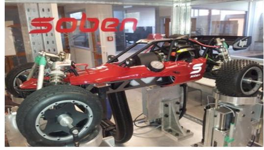
Fig. 3. SOBEN Semi-active suspension platform
