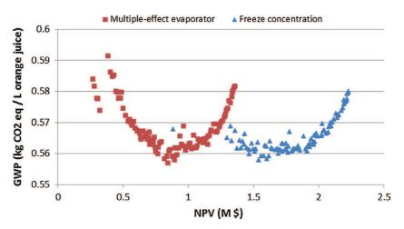
Fig. 9. NPV and GWP 2D Pareto front output for Sc3 with Concentration Technology Selection variable.
